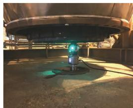
0.0006in) align and verify centerline alignment for any piece of rotating or reciprocating equipment with record speed. The Faro Tracker system is extremely versatile when time is of the essence. Real-time 3 dimensional readings can be displayed when internal components
